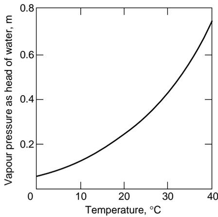
FIG. 9.20. Vapour pressure of water as head (m) versus temperature.
