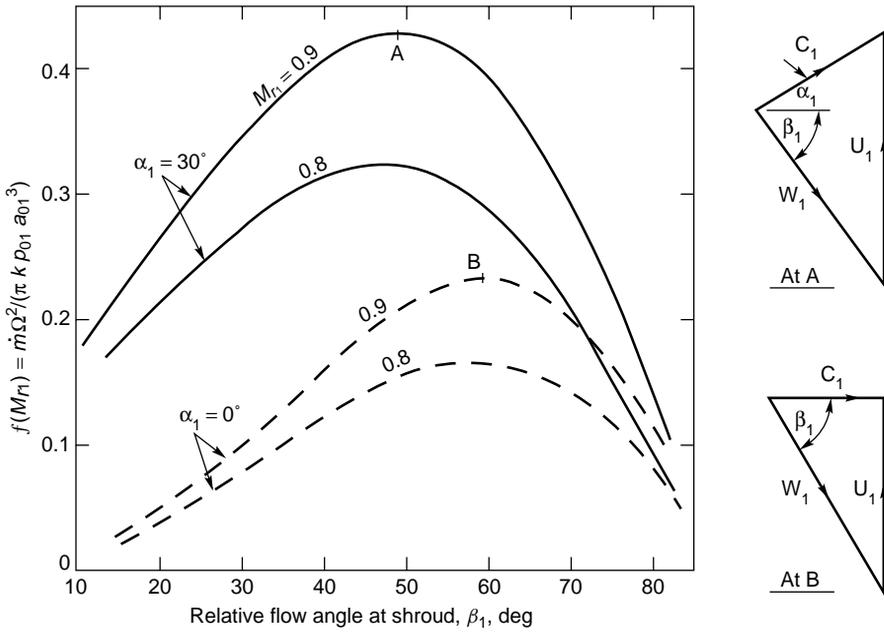
FIG. 7.4. Variation of mass flow function for the inducer of a centrifugal compressor with and without guide vanes ( $\gamma = 1.4$ ). For comparison both velocity triangles are drawn to scale for  $M_{r1} = 0.9$  the peak values or curves.
