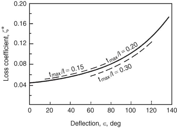
FIG. 4.3. Soderberg's correlation of turbine blade loss coefficient with fluid deflection (adapted from Horlock (1960)).
