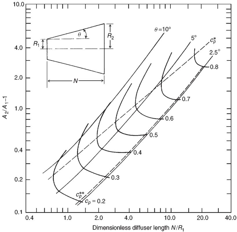
FIG. 2.17. Performance chart for conical diffusers,  $B_1 \cong 0.02$ . (adapted from Sovran and Klomp 1967).
