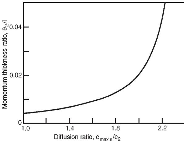
FIG. 3.17. Mean variation of wake momentum-thickness/chord ratio with suction-surface diffusion ratio at reference incidence condition for NACA 65 - (C<sub>10</sub>A<sub>10</sub>)10 blades and British C.4 circular-arc blades (adapted from Lieblein (1959)).
