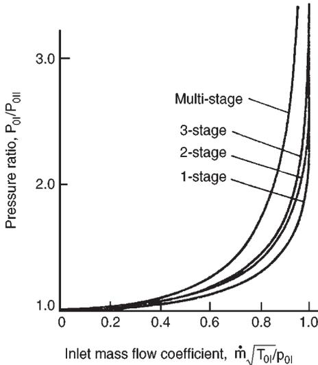
FIG. 4.21. Turbine flow characteristics (after Mallinson and Lewis 1948).
