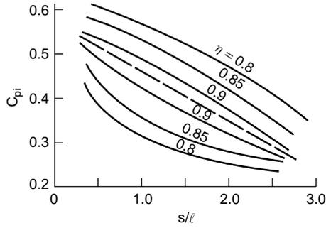
FIG. 3.23. Efficiency correlation (adapted from McKenzie 1988).
