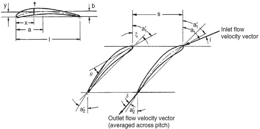
FIG. 3.2. Compressor cascade and blade notation.
