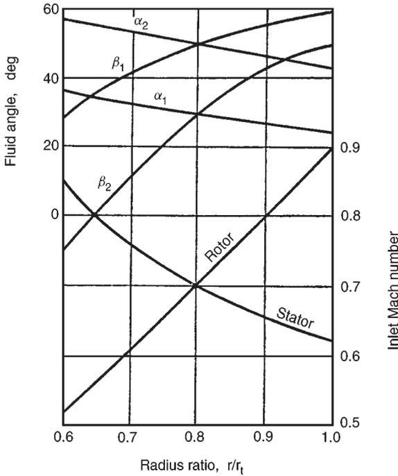
FIG. 6.4. Variation of fluid angles and Mach numbers of a free-vortex compressor stage with radius (adapted from Howell 1945).
