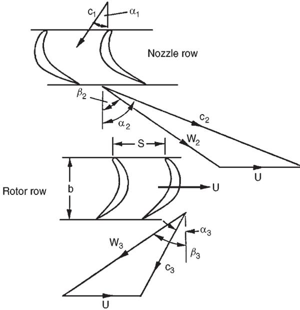
FIG. 4.1. Turbine stage velocity diagrams.
