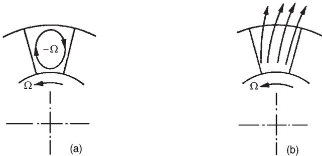
FIG. 7.8. (a) Relative eddy without any throughflow. (b) Relative flow at impeller exit (throughflow added to relative eddy).
