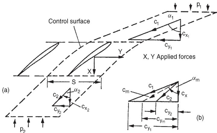
FIG. 3.3. Forces and velocities in a blade cascade.
