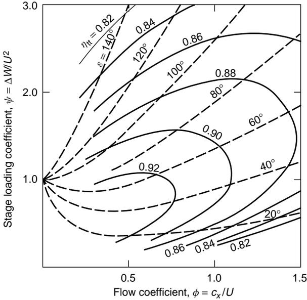
FIG. 4.10. Design point total-to-total efficiency and deflection angle contours for a turbine stage of 50 per cent reaction.
