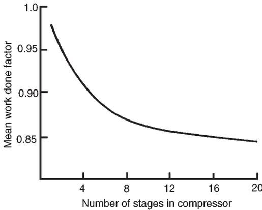
FIG. 5.9. Mean work done factor in compressors (Howell and Bonham 1950). (Courtesy of the Institution of Mechanical Engineers).
