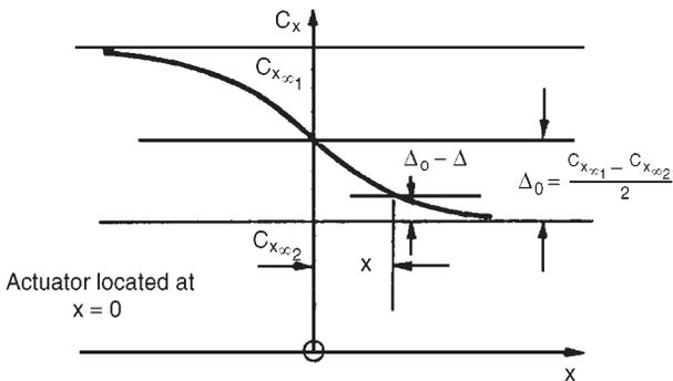
FIG. 6.12. Variation in axial velocity with axial distance from the actuator disc.
