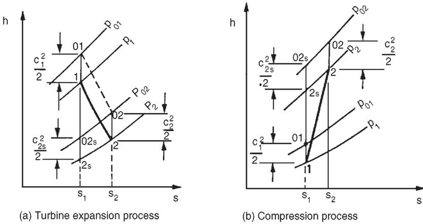
FIG. 2.5. Enthalpy-entropy diagrams for turbines and compressors.
