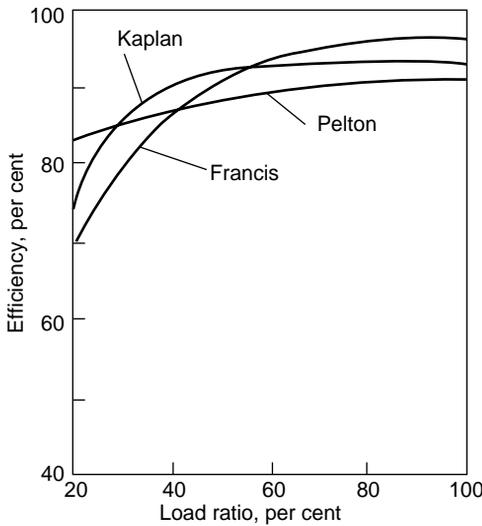
FIG. 9.14. Variation of hydraulic efficiency for various types of turbine over a range of loading, at constant speed and constant head.
