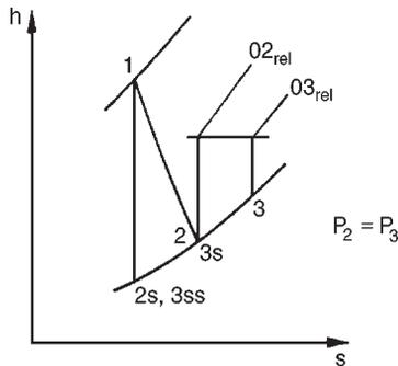
FIG. 4.6. Mollier diagram for an impulse turbine stage.
