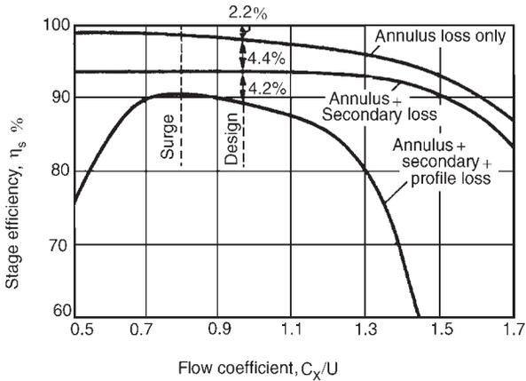
FIG. 3.13. Losses in a compressor stage (Howell 1945). (Courtesy of the Institution of Mechanical Engineers).
