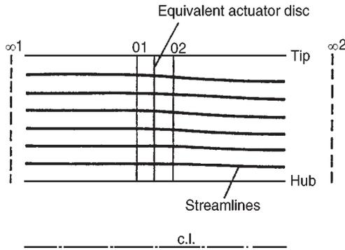
FIG. 6.11. The actuator disc assumption (after Horlock 1958).
