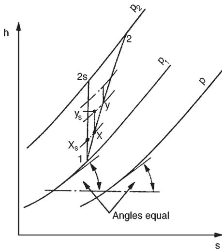
FIG. 2.6. Compression process by small stages.
