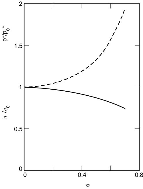
FIG. 4.27. Variation of peak efficiency and non-dimensional pressure drop (in comparison to the values for an isolated aerofoil) vs solidity: - - - pressure \_\_\_\_\_ efficiency (adapted from Raghunathan *et al.* 1995).
