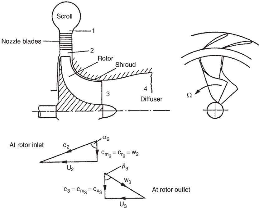
FIG. 8.3. Layout and velocity diagrams for a 90 deg inward flow radial turbine at the nominal design point.
