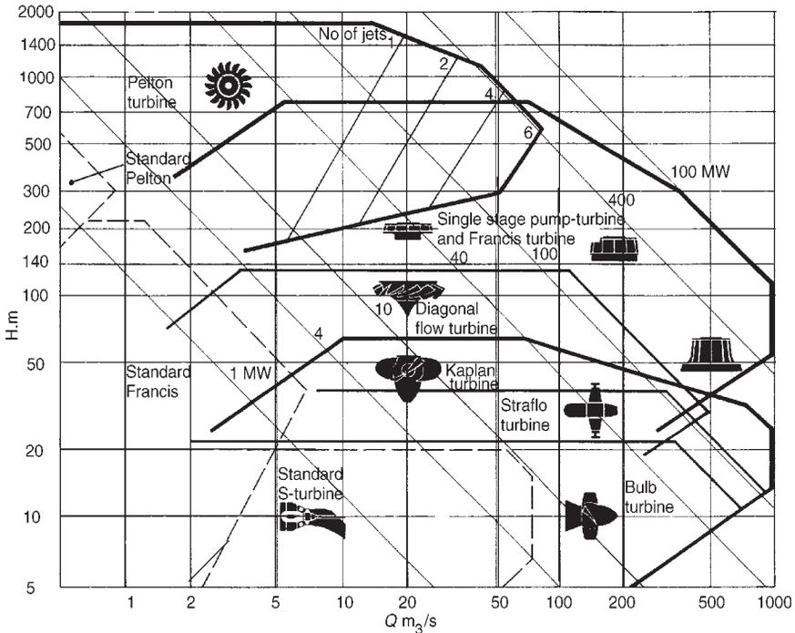
FIG. 9.2. Application ranges for various types of hydraulic turbomachines, as a plot of  $Q$  vs  $H$  with lines of constant power determined assuming  $\eta_0 = 0.8$ . (Courtesy Sulzer Hydro Ltd., Zurich).
