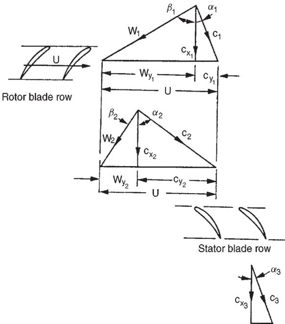
FIG. 5.2. Velocity diagrams for a compressor stage.
