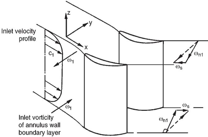
FIG. 6.15. Secondary vorticity produced by a row of guide vanes.
