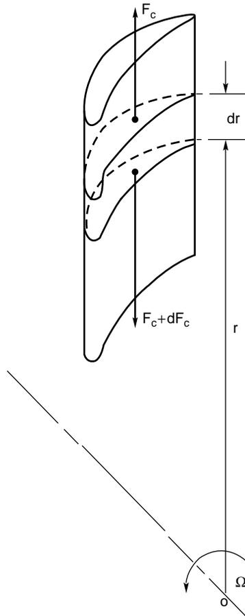
FIG. 4.15. Centrifugal forces acting on rotor blade element.
