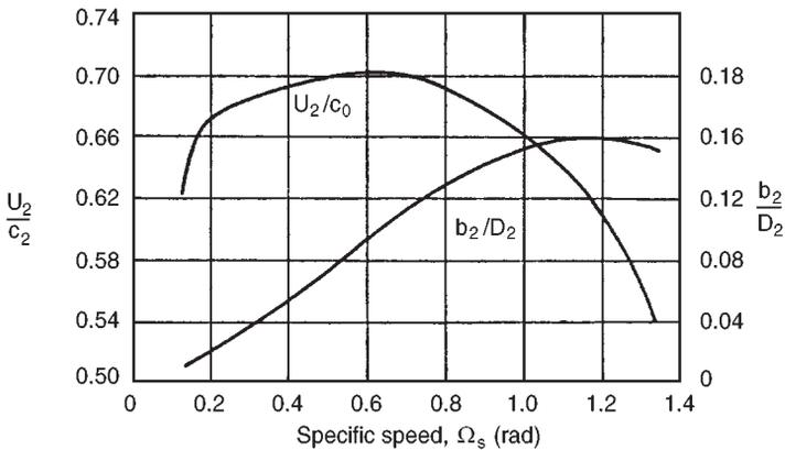
FIG. 8.17. Variation in blade speed/spouting velocity ratio ( $U_2/c_0$ ) and nozzle blade height/rotor inlet diameter ( $b_2/D_2$ ) corresponding to maximum total-to-static efficiency with specific speed (adapted from Rohlik 1968).
