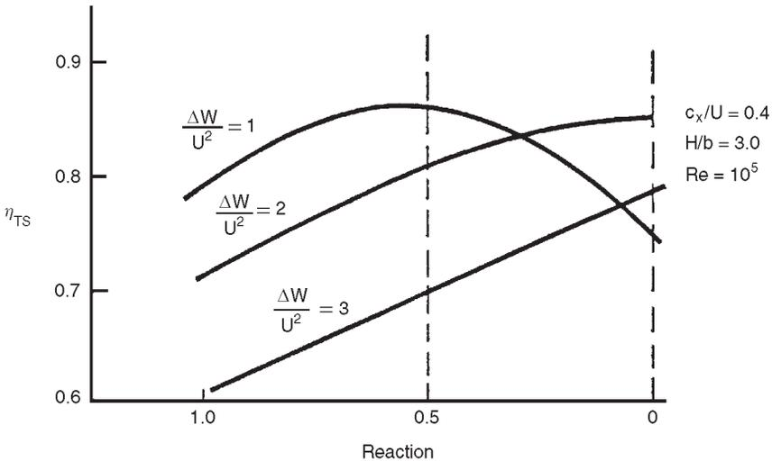
FIG. 4.9. Influence of reaction on total-to-static efficiency with fixed values of stage loading factor.
