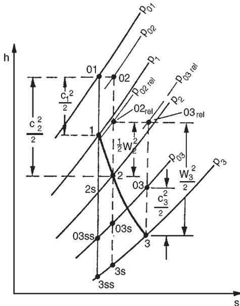
FIG. 4.2. Mollier diagram for a turbine stage.
