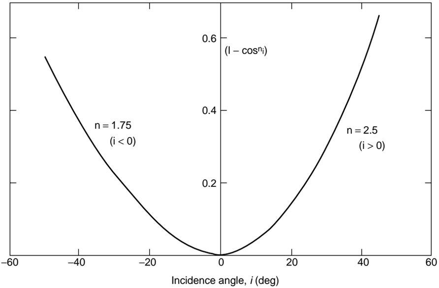
FIG. 8.11. Variation of incidence loss function at rotor inlet as a function of the incidence angle.
