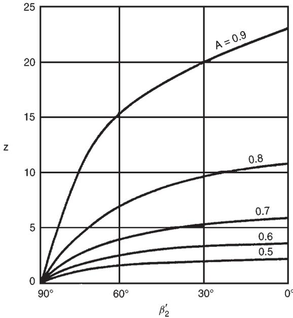
FIG. 7.11. Head correction factors for centrifugal impellers (adapted from Csanady (1960)).
