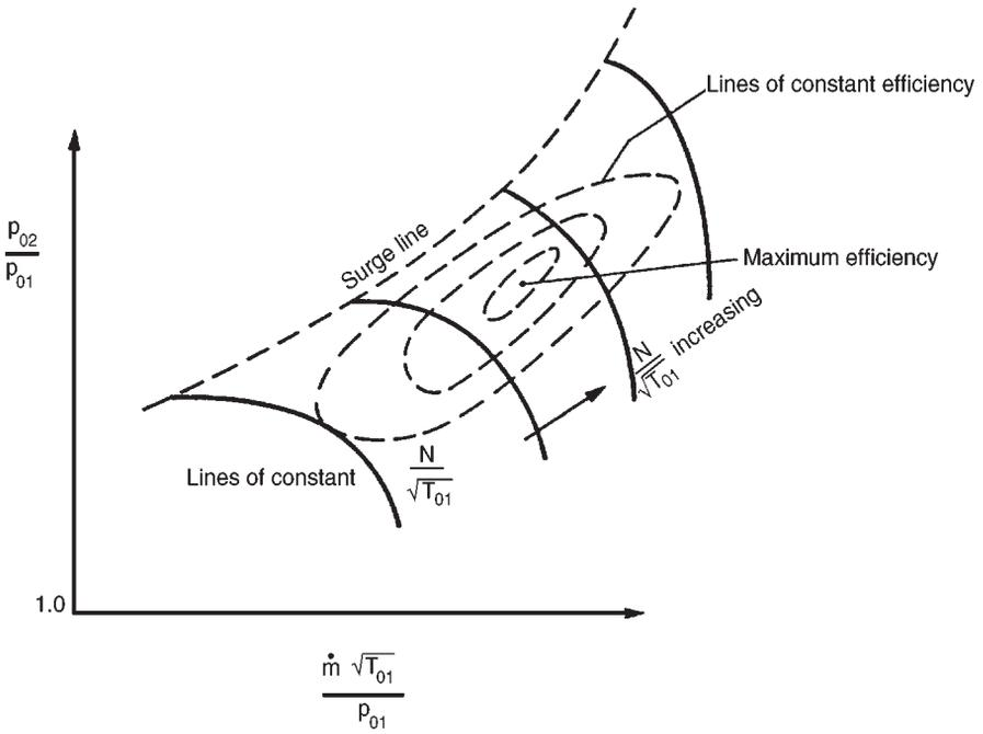
FIG. 1.10. Overall characteristic of a compressor.
