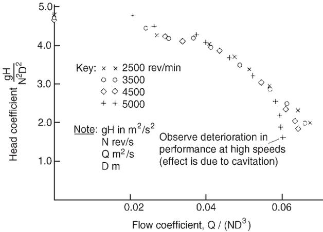
FIG. 1.3. Dimensionless head-volume characteristic of a centrifugal pump.
