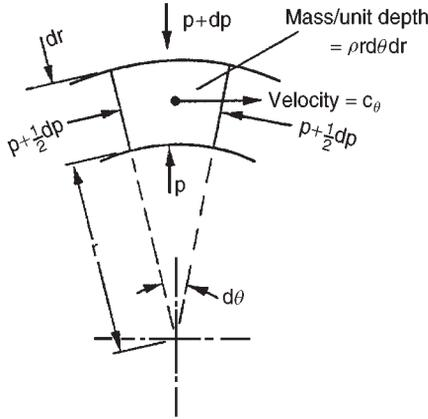
FIG. 6.2. A fluid element in radial equilibrium ( $c_r = 0$ ).
