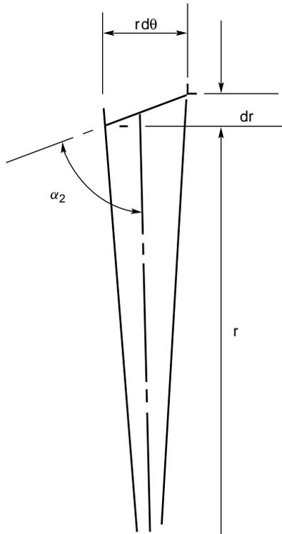
FIG. 7.15. Element of flow path in radial diffuser.
