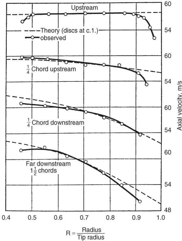
FIG. 6.9. Variation of the distribution in axial velocity through a row of guide vanes (adapted from Hawthorne and Horlock 1962).
