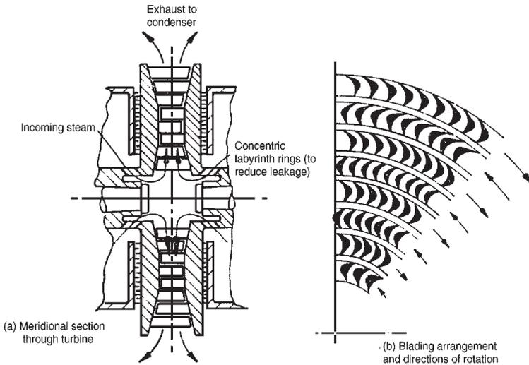
FIG. 8.1. Ljungström type outward flow radial turbine (adapted from Kearton<sup>(2)</sup>).
