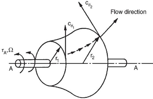
FIG. 2.4. Control volume for a generalised turbomachine.
