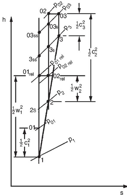
FIG. 5.3. Mollier diagram for an axial compressor stage.
