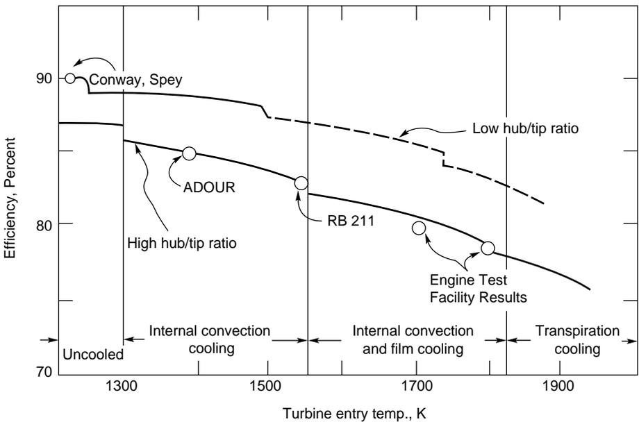
FIG. 4.20. Turbine thermal efficiency vs inlet gas temperature (adapted from le Grivès 1986).
