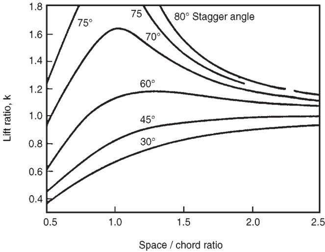
FIG. 5.16. Weing's results for lift ratio of a cascade of thin flat plates, showing dependence on stagger angle and space/chord ratio (adapted from Wislicenus (1947)).
