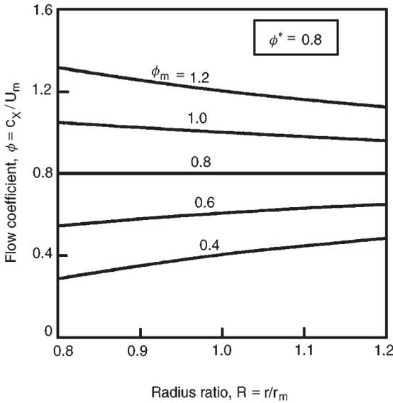
FIG. 6.8. Off-design rotor exit flow coefficients.
