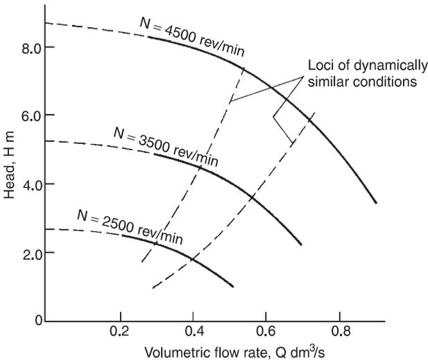
FIG. 1.4. Extrapolation of characteristic curves for dynamically similar conditions at  $N = 3500$  rev/min.
