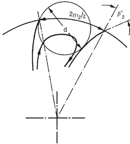
FIG. 7.9. Flow model for Stodola slip factor.
