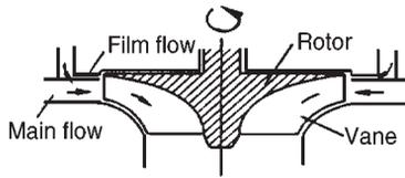
FIG. 8.19. Cross section of film-cooled radial turbine.
