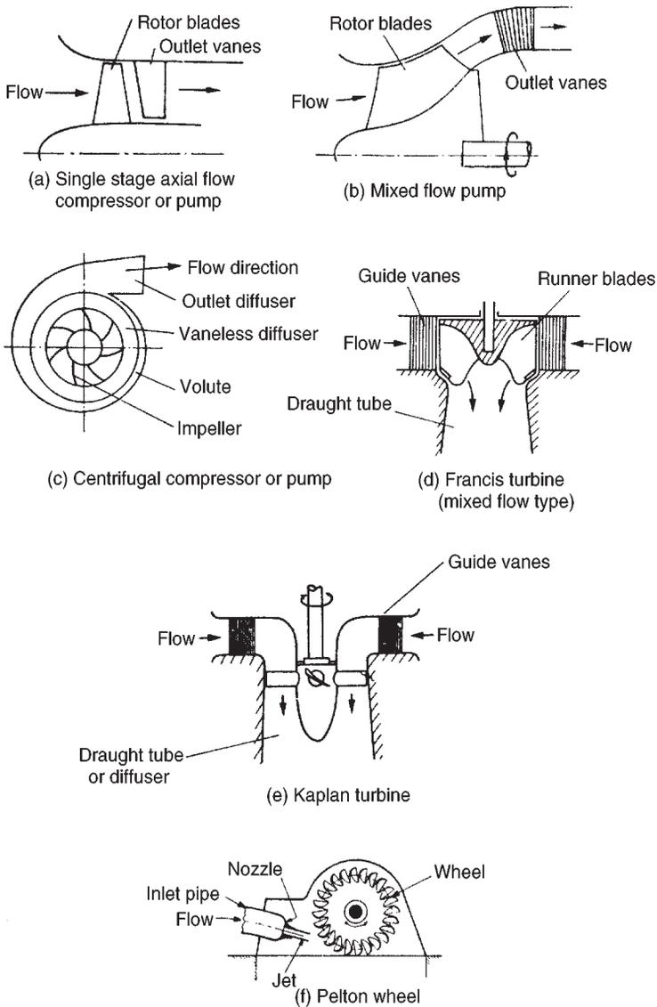
FIG. 1.1. Diagrammatic form of various types of turbomachine.
