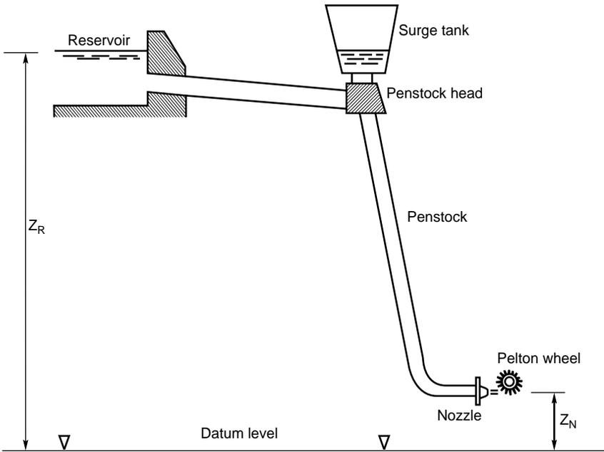
FIG. 9.7. Pelton turbine hydroelectric scheme.
