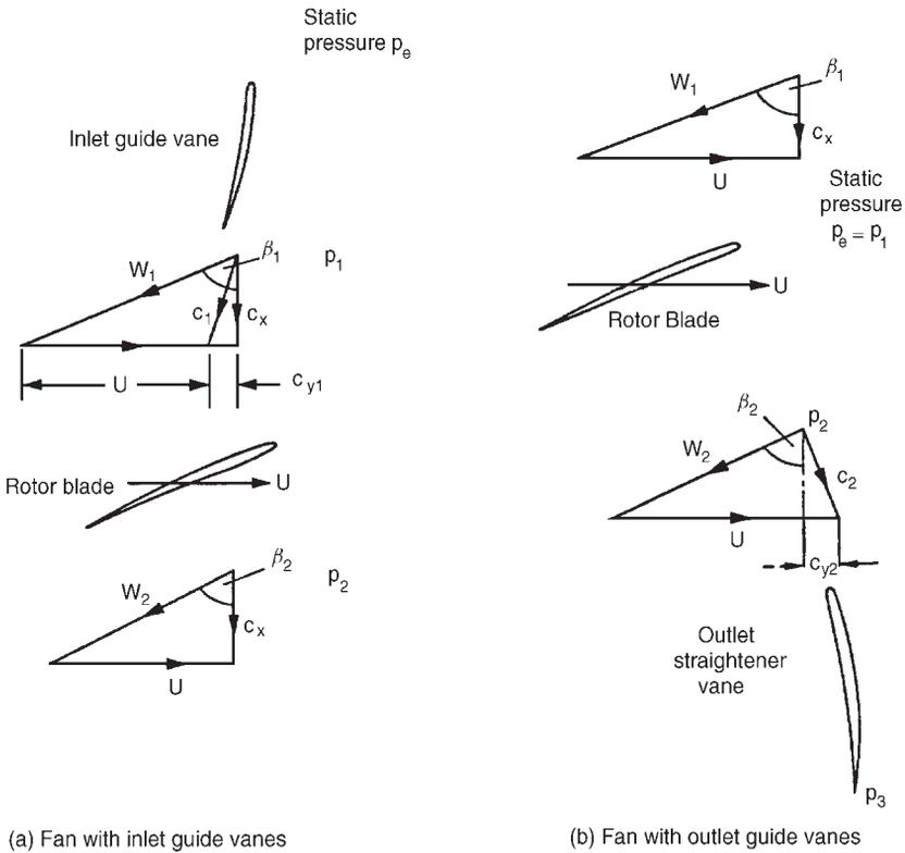
FIG. 5.17. Two simple types of axial-flow fan and their associated velocity diagrams (after Van Niekerk 1958).
