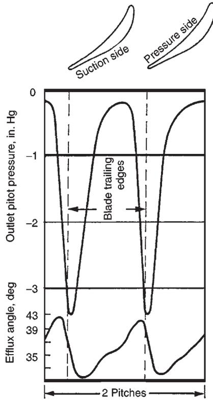
FIG. 3.11. A sample plot of inlet and outlet stagnation pressures and fluid outlet angle (adapted from Todd 1947).
