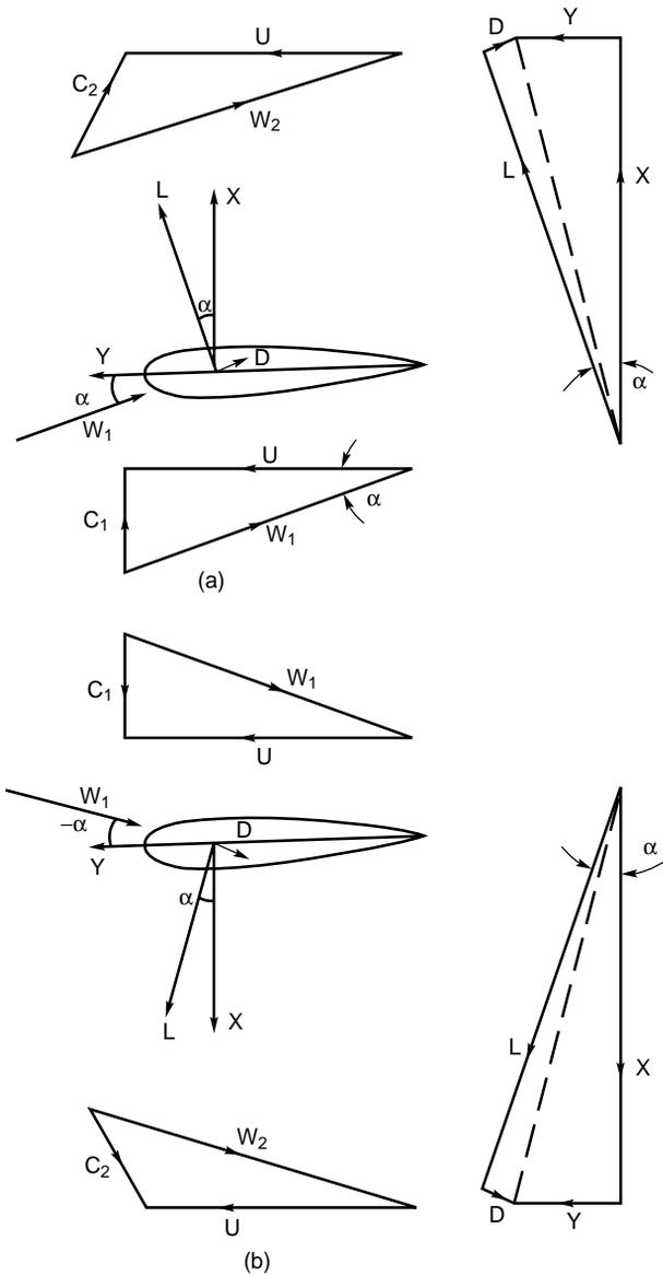
FIG. 4.25. Velocity and force vectors acting on a blade of a Wells turbine in motion: (a) upward absolute flow onto blade moving at speed  $U$ ; (b) downward absolute flow onto blade moving at speed  $U$ .
