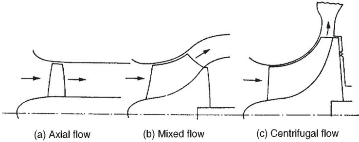
FIG. 1.7. Range of pump impellers of equal inlet area.
