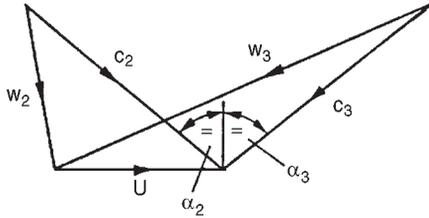
FIG. 4.8. Velocity diagram for 100% reaction turbine stage.
