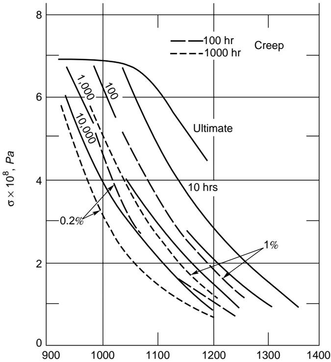
FIG. 4.18. Properties of Inconel 713 Cast (adapted from Balje 1981).
