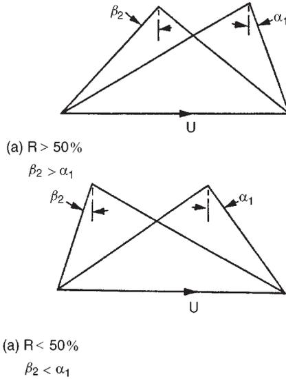
FIG. 5.4. Asymmetry of velocity diagrams for reactions greater or less than 50%.
