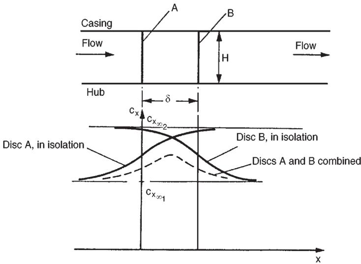
FIG. 6.13. Interaction between two closely spaced actuator discs.
