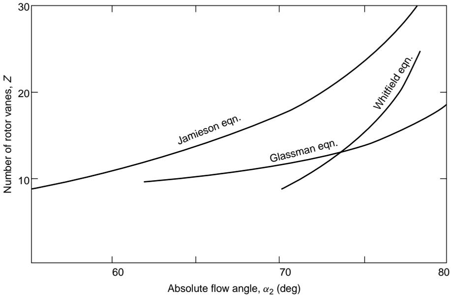
FIG. 8.7. Flow angle at rotor inlet as a function of the number of rotor vanes.
