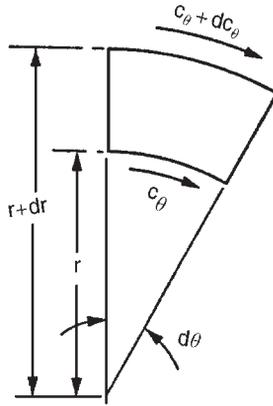
FIG. 6.3. Circulation about an element of fluid.
