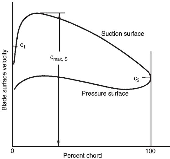
FIG. 3.15. Compressor cascade blade surface velocity distribution.
