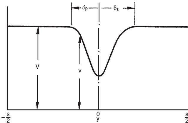
FIG. 3.16. Model variation in velocity in a plane normal to axial direction.
