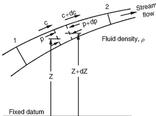
FIG. 2.3. Control volume in a streaming fluid.
