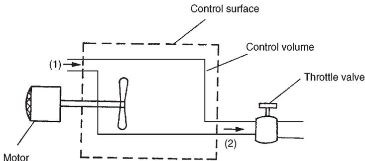
FIG. 1.2. Turbomachine considered as a control volume.
