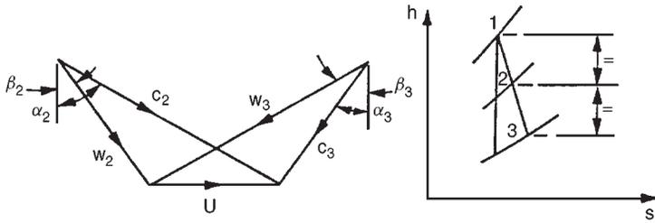
FIG. 4.7. Velocity diagram and Mollier diagram for a 50% reaction turbine stage.
