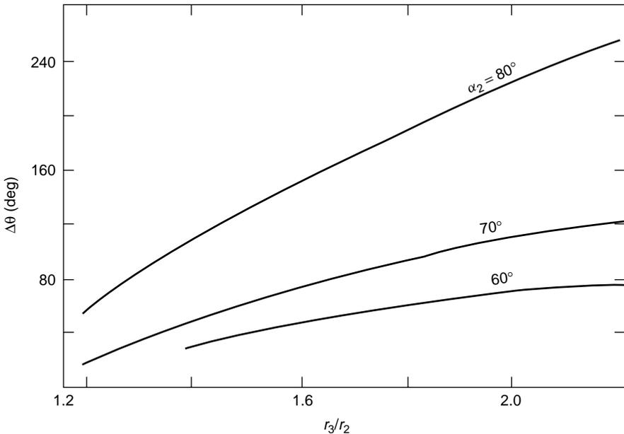
FIG. 7.16. Flow path data for parallel-walled radial diffuser (incompressible flow).
