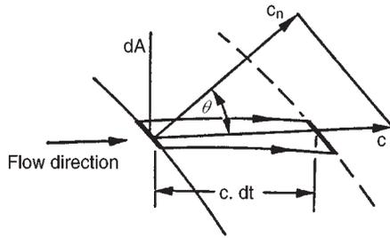
FIG. 2.1. Flow across an element of area.
