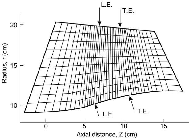
FIG. 6.14. Typical computational mesh for a single blade row (adapted from Macchi 1985).
