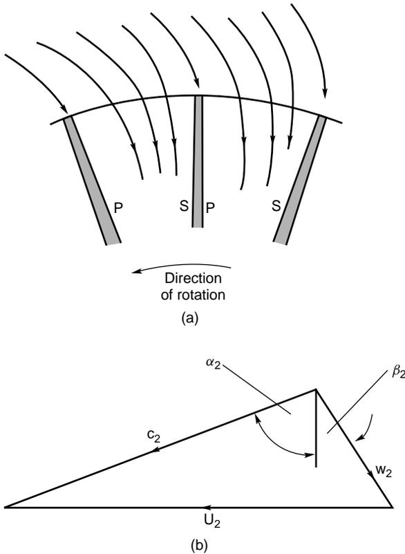
FIG. 8.5. Optimum flow condition at inlet to the rotor. (a) Streamline flow at rotor inlet; p is for pressure surface, s is for suction averaged flow. (b) Velocity diagram for the pitchwise averaged flow.
