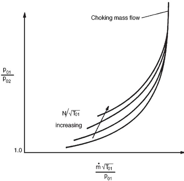
FIG. 1.11. Overall characteristic of a turbine.
