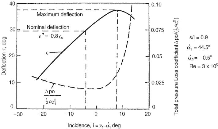
FIG. 3.12. Compressor cascade characteristics (Howell 1942). (By courtesy of the Controller of H.M.S.O., Crown copyright reserved).
